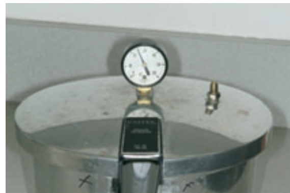
Figure 40. Models placed in a pressure pot for 10 minutes. (Color version of figure is available online.)
