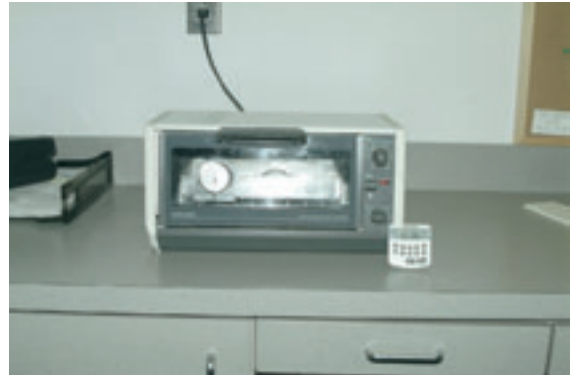
Figure 26. Thermally cured resins can also be used to create custom bases and are cured in a toaster oven at 325°F for 15 minutes. (Color version of figure is available online.)
